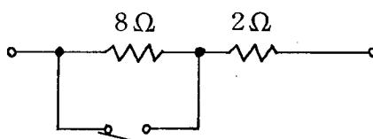
$$\left\{ \begin{array}{l} \text{スイッチ ON } \underline{\hspace{2cm}} \quad [\Omega] \\ \text{スイッチ OFF } \underline{\hspace{2cm}} \quad [\Omega] \end{array} \right.$$
