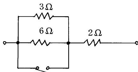
$$\left\{ \begin{array}{l} \text{スイッチ ON } \underline{\hspace{2cm}} \quad [\Omega] \\ \text{スイッチ OFF } \underline{\hspace{2cm}} \quad [\Omega] \end{array} \right.$$
